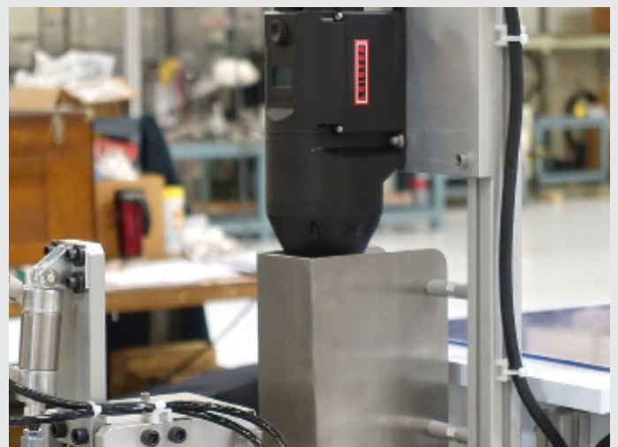
Leister MISTRAL hot-air blower installed in a production system.
